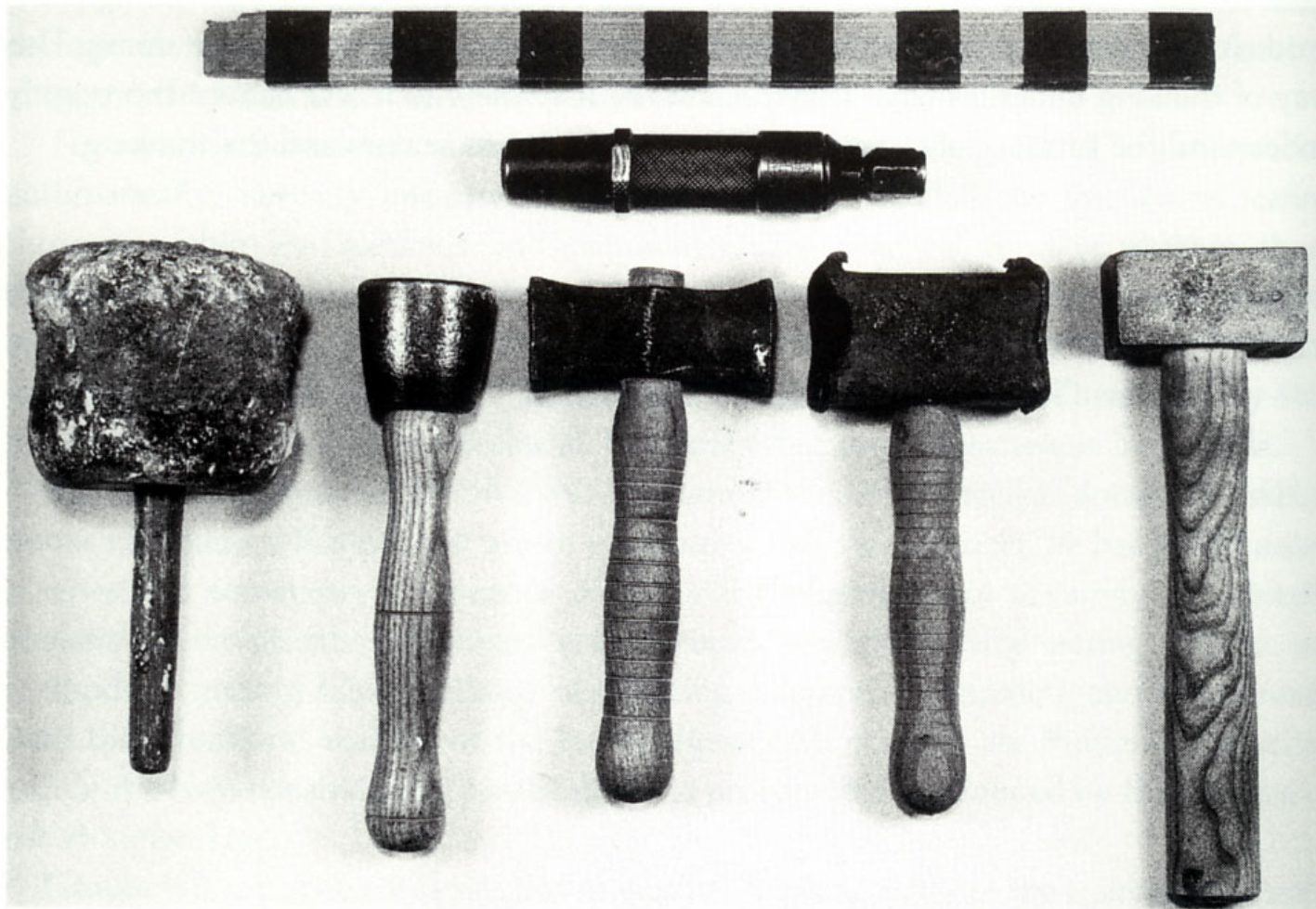
2. Hammers: (from left to right) an American mallet, a French metal mallet, two Italian hammers, an English finishing hammer. At the top is an air hammer.
