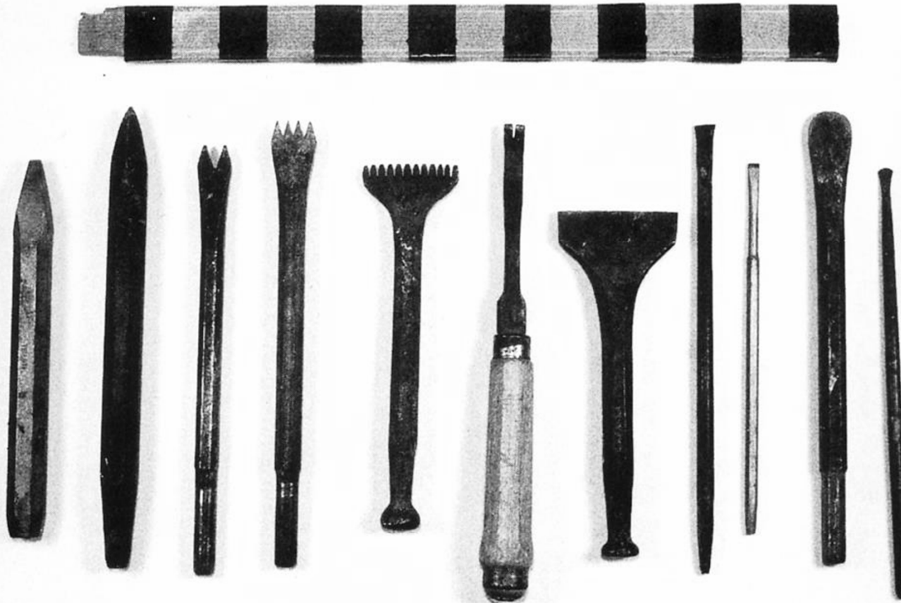
3. Carving tools: (from left to right) a granite point chisel, a marble point chisel, two tooth chisels for the air hammer, two tooth chisels for a wooden mallet, a flat chisel for a wooden mallet, two flat chisels for a metal hammer, a round-headed chisel for the air hammer, a round-headed chisel for a metal hammer.
