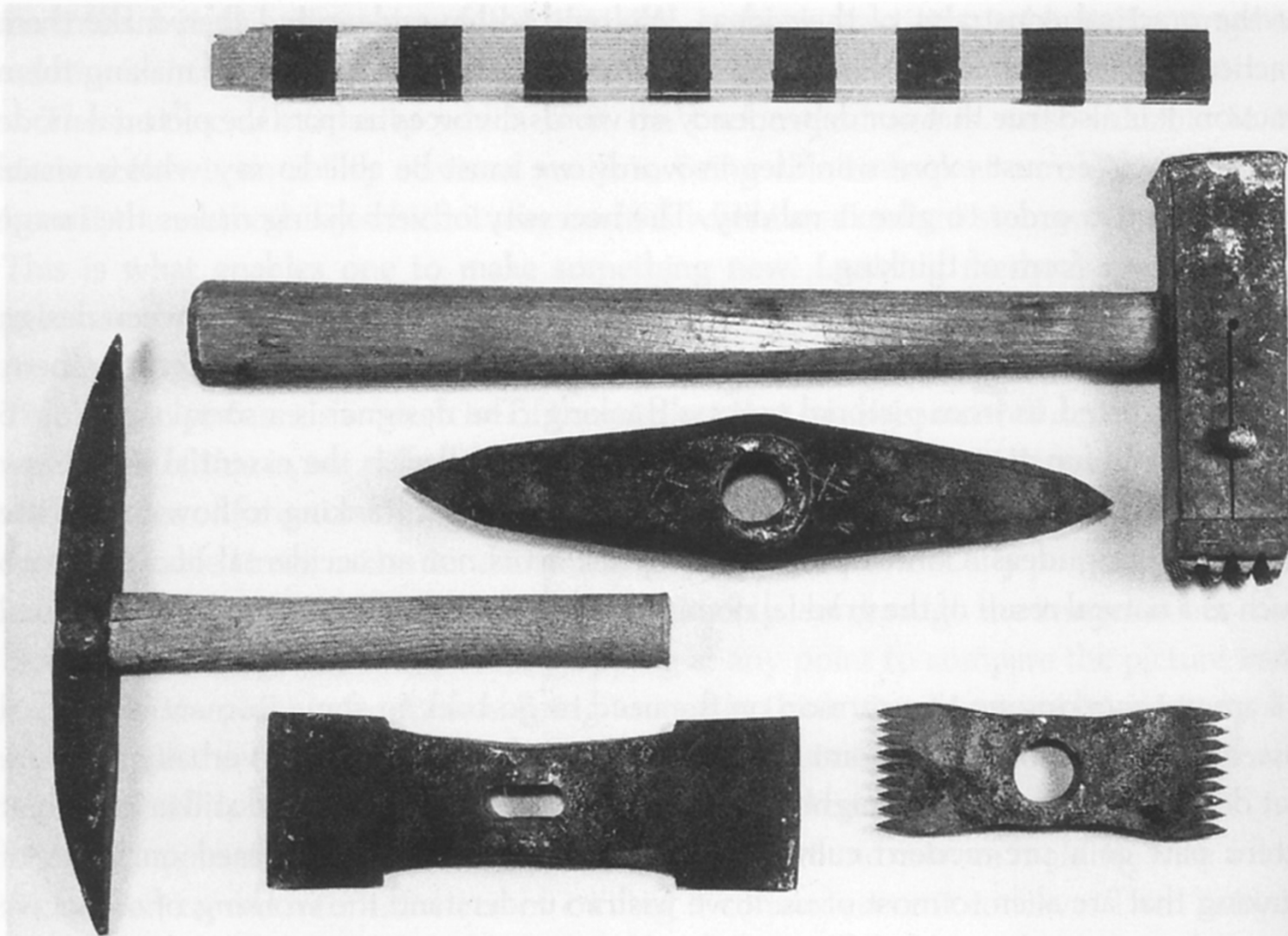
1. Axes: (from lower left to upper right) an Italian sculptor's pick, two Italian mason's axeheads, a Turkish quarry pick, an Italian bush hammer.
